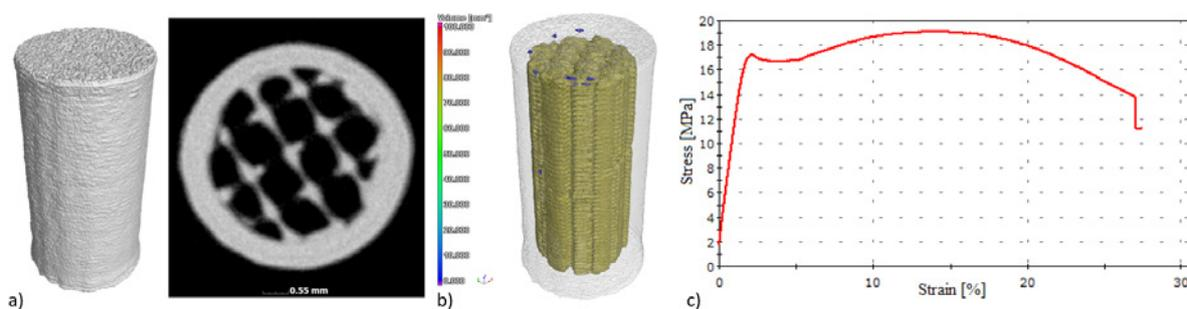
Fig. 1a), b) The result of CT reconstruction – 2D and 3D view, c) Stress-strain curve
