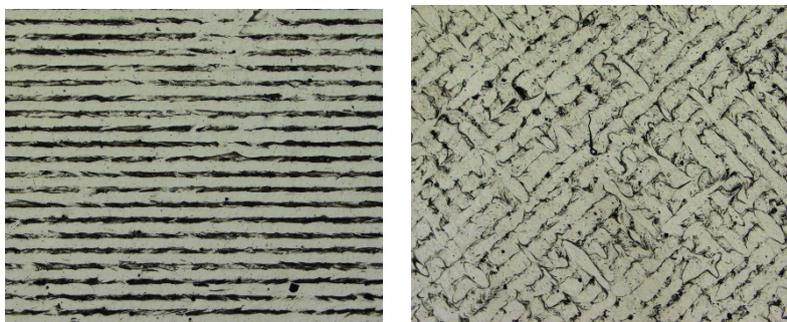
Fig. 1. Examples of crystalline (dark) – amorphous (white) composites obtained in the process
