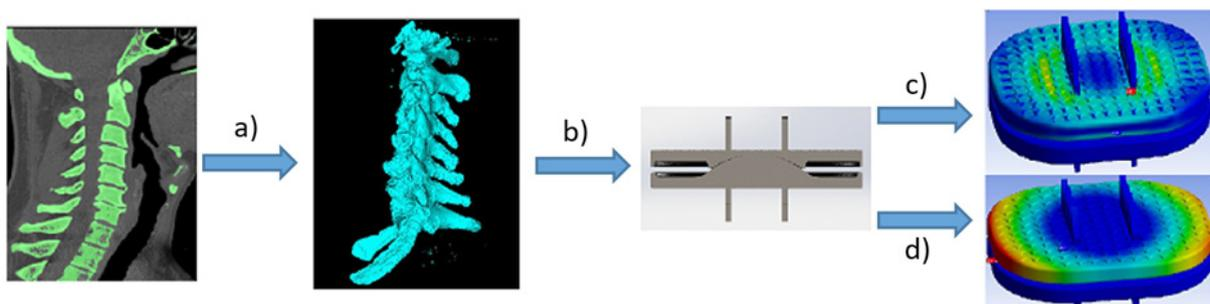
Fig. 1. The process of designing personalized product: a) obtain the geometry of vertebrae, b) modeling the implant geometry, c) maximum strength in the FEM simulation, d) maximum deformations in the FEM simulation
