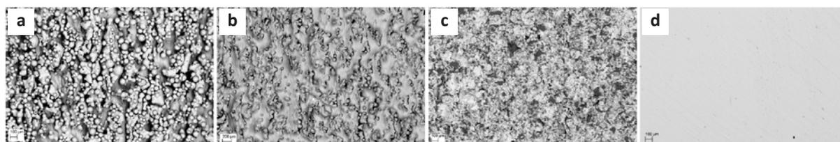
Fig.1. The result of surface modification processes: a) as build, b) acid-etched, c) sandblasted, d) machined, SEM
