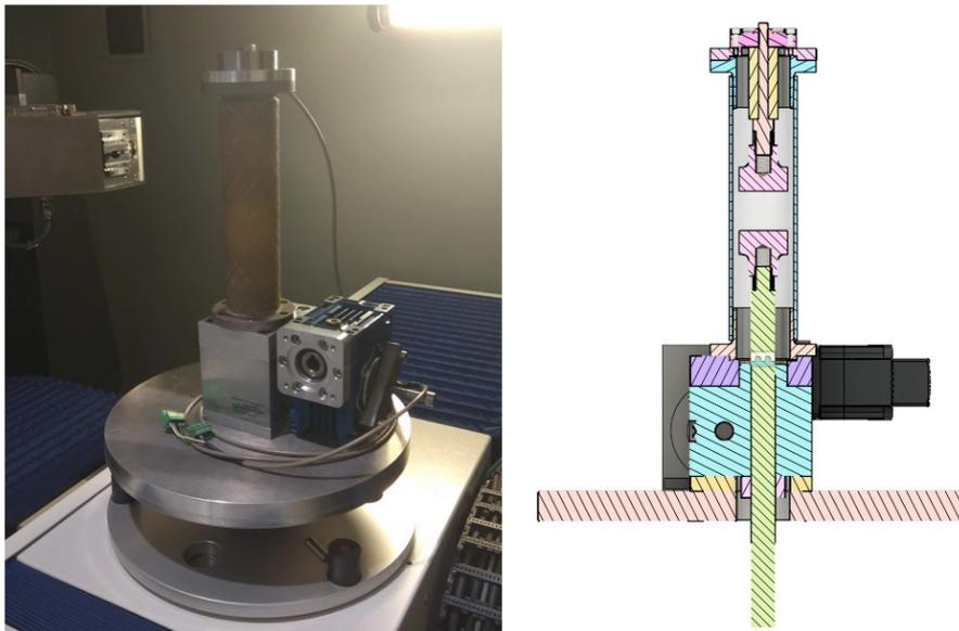
Fig. 1. Test device concept: adjustment in the CT (left) and scheme (right).
